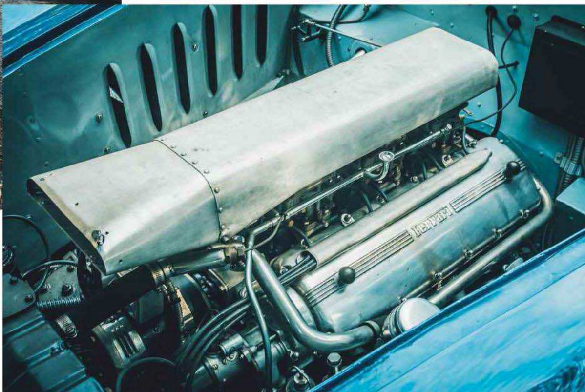
Above and right Engineer Colombo's original 1.5-litre V12 had grown to 2.34 litres by 1951 (195 referring to the cubic capacity of each cylinder). This 195 Inter has the triple Webers of the Sport model
